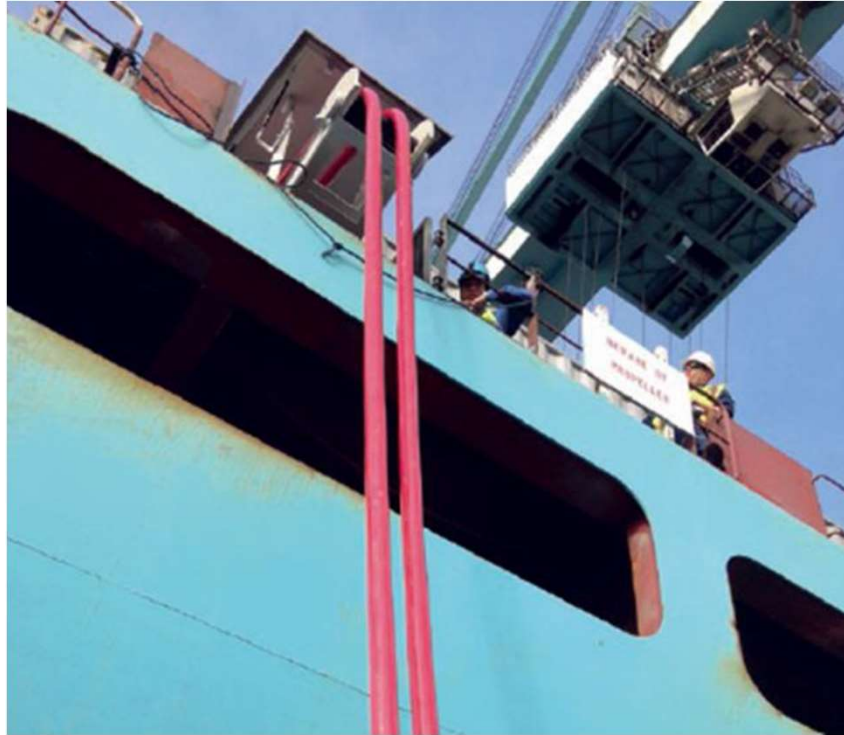
SSE cables from MAESK container ship (Maersk Line, 2014)
